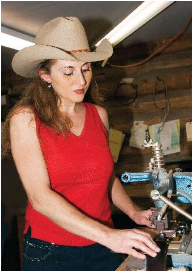
Everyone in the shop can perform multiple jobs but each has a specialty. Here, Shama uses heat transfer to stamp the owner's name on a sweatband with 23-karat gold foil.
